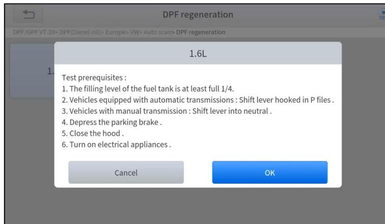
4. Read the fuel tank level and make sure that it fulfills the requirement displayed.
