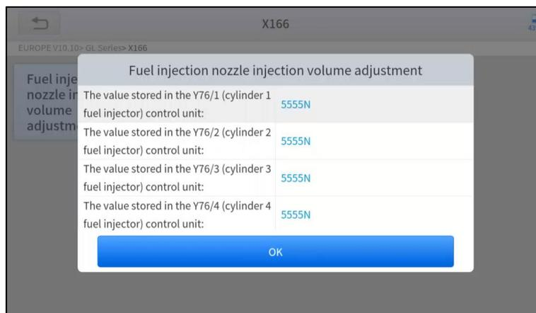
5. Enter the **Change the value of cylinder** menu of the replaced injector(s), enter the **new 5-digit value**, and then press **OK**.
