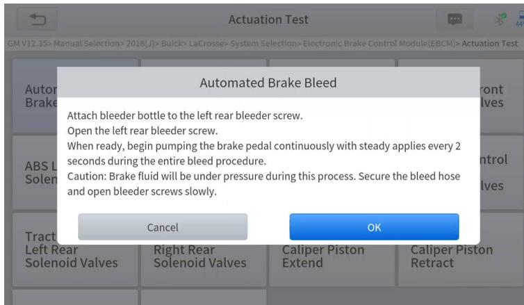
4. When ready, click "**OK**" to enter the bleed procedure, and pumping the brake pedal continuously with steady applies every 2 seconds during the entire procedure
