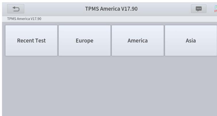
TPMS reset can be further divided into 4 methods, such as **Automatic Relearn, Static Relearn, Copy ID and OBD Relearn**, which is depending on the specific model. Also, even if the relearning methods are the same, the learning procedure may differ.
