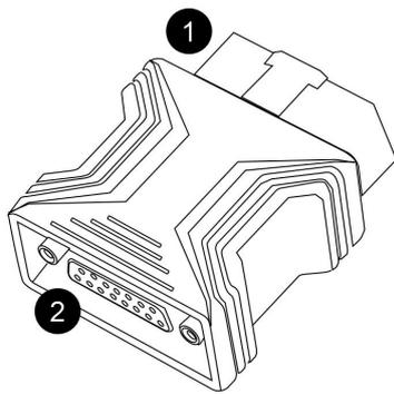
1. OBD Male Connector – Plug into vehicle's DLC port
